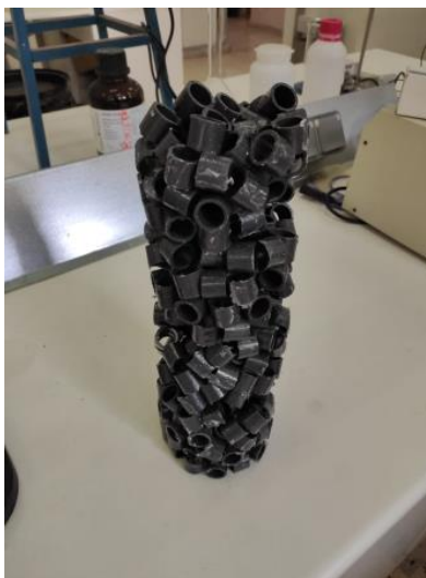
Figure 2. Packed bed structure.
