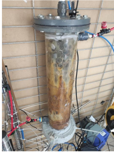
Figure 23. Biotrickling filter under maximum elimination capacity.
